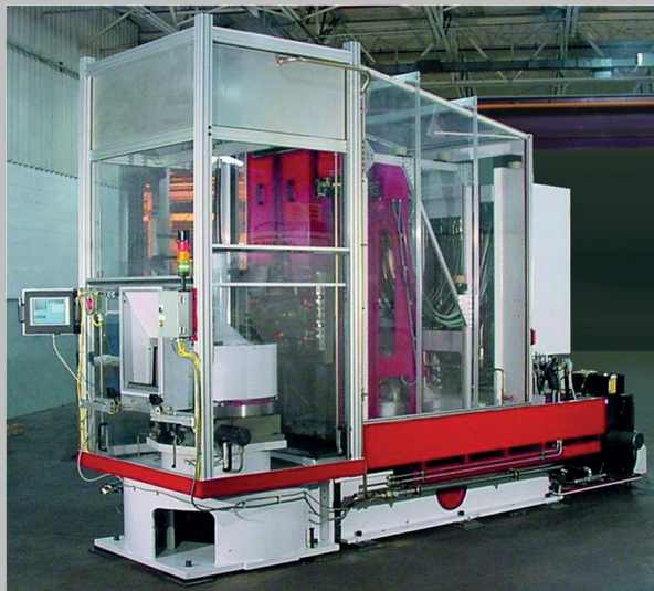
Figure 26. My detour. The flexible adaptive servo-hydraulic technology (FAST) machine tool I designed at my dad's company.
